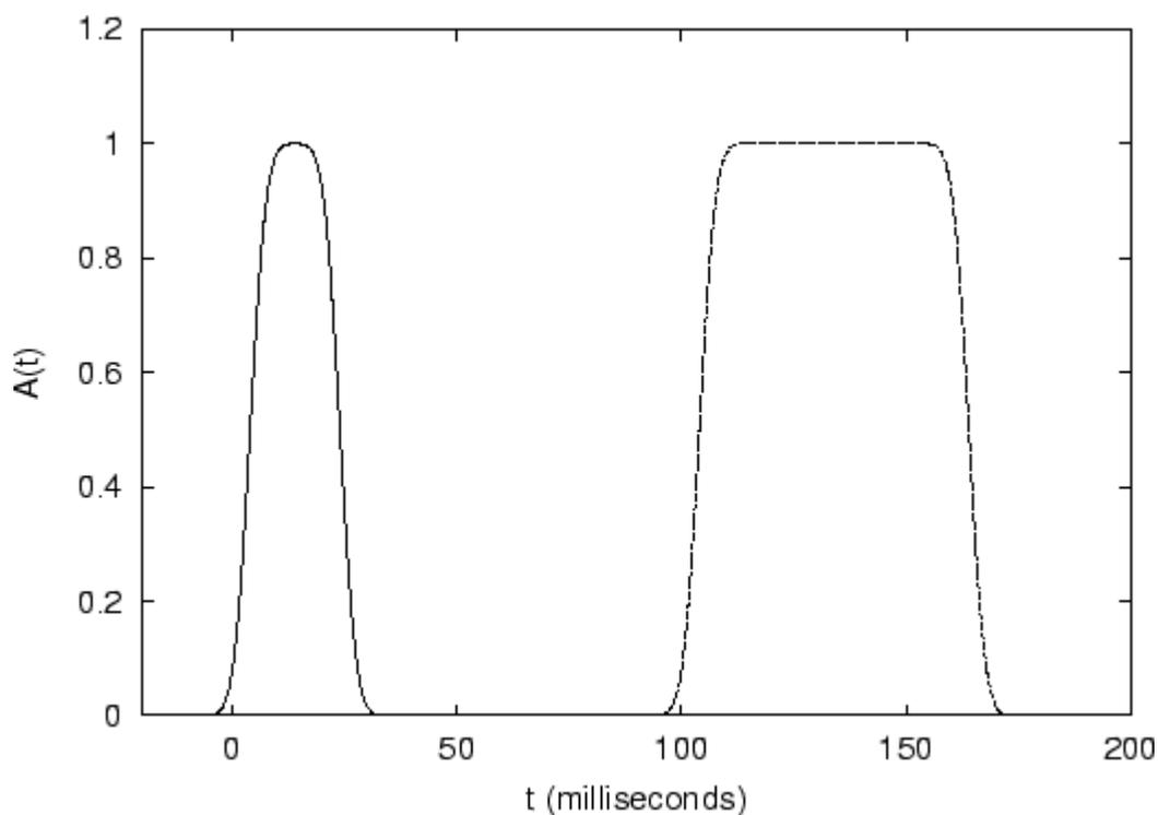
**Figure 6:** The error function keying waveforms for  $\tau$  of 4 milliseconds and durations of 20 and 50 milliseconds. The 50 millisecond pulse begins at  $t = 100$  milliseconds to separate it from the 20 millisecond pulse.
