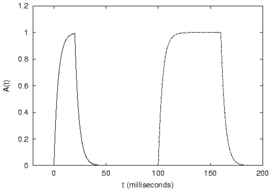
**Figure 1:** The exponential keying waveforms for a time constant  $\tau$  of 4 milliseconds and durations of 20 and 50 milliseconds. The 50 millisecond pulse begins at  $t = 100$  milliseconds to separate it from the 20 millisecond pulse.
