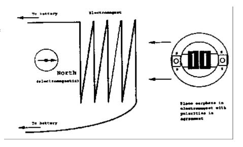
and diaphragm from the weak earphone and place it inside the electromagnet winding with the poles of the electromagnet and the earphone matching (both north poles to the left etc.) Connect the winding to the cell, in the same manner, tap, tap, tap. Do it about 6 times. Check the earphone polarity. It should be the same as you marked it. Check it with the diaphragm for hanging strength. It should be much stronger.
