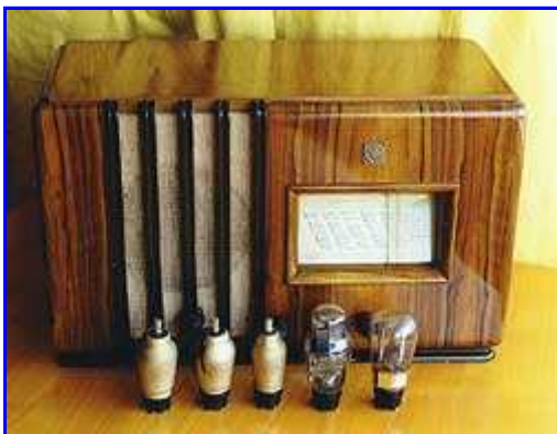
A 1938 Telefunken table-model radio. Note: tubes have side-contacts, not pins. [All photos by the author.]
