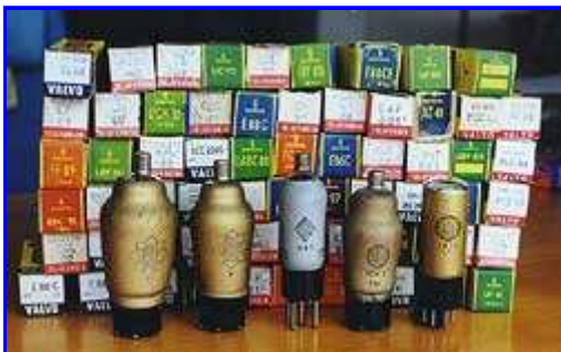
European tubes from more than five decades of production can be identified using the schemes explained in the tables.
