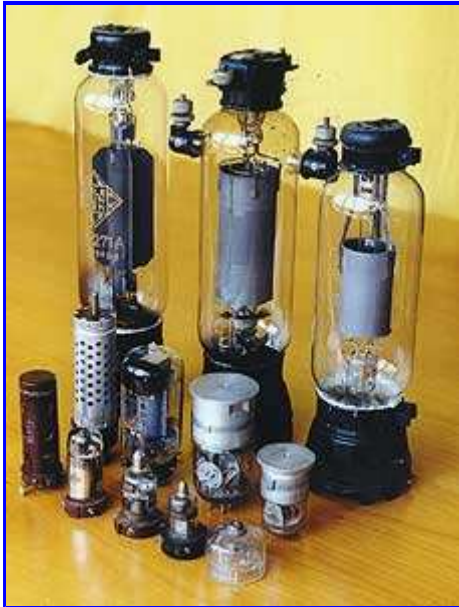
Military tubes from the 1930s and 1940s. All have special bases and sizes because of miniaturization and high-frequency requirements. The tall transmitting tubes use Telefunken tube code.
