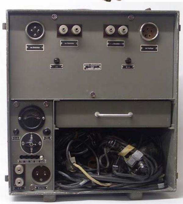
The receiver can be powered from 6V accumulators or from the mains. The 6V DC voltage is used directly for valve heaters and via a "Mallory vibrator" to generate the B+ voltage of 120V which will be rectified again.
