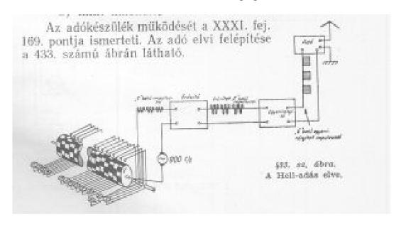
At reception, the transmitted telegraph signals are transmitted to the radio through the receiving antenna, and then the amplification and rectification of the incoming frequency is already done in HTG-1. The writer consists of an electromagnet, the tongue of which presses the continuous web of tape onto the rotating spindle. This will display a letter or punctuation mark on the tape.
