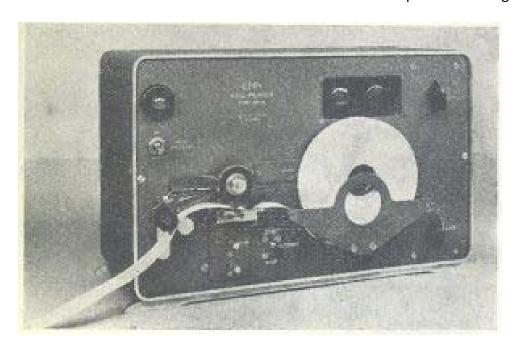
The 49 M HTG-1 transmitter is a vibration-generating tube - it produces 900-wave waves. The transmitter also includes a contact roll and a key system.
