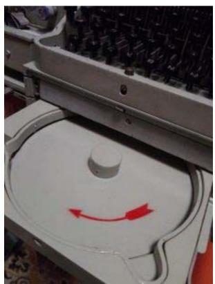
The circumference of the cylinder, as shown in the figure, is also divided into forty-nine slices - and each character and letter has its own code. By pressing the letters, the mechanics push the corresponding scanner onto the surface of the continuously rotating cylinder, where the spring closes the metal to the metal surface and opens it on the insulated. Through the contacts, the signals of the vibration generator 6BA6 are partly transmitted to the line and partly to the receiver itself.
