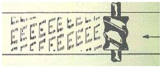
If the transmitter and receiver machine speed is different, the written text will be inclined. If the transmitter is in a hurry, the rows will move from left to right if slower, from left to right.
