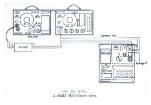
In the above figure, it is worth noting that although it is from a 1952 book, it can be seen on the German Feld Hell and an R / 7 transmitter and R / 7 receiver.
