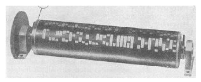
Transmission is done by pressing the appropriate lever on a typewriter keyboard. The Hell machine recorder, as described above, is a rhythmic system, which means that it can only be written on a regular basis. Its speed is 150 letters per minute.
