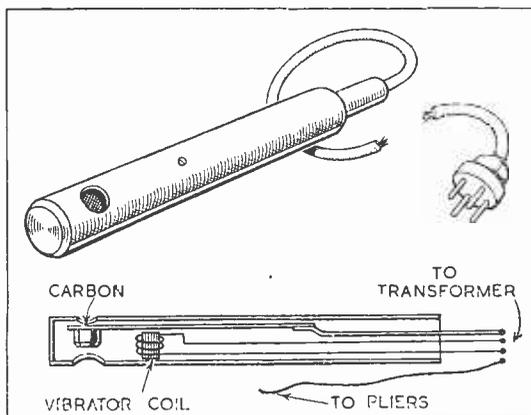
by one inch in diameter. The vibro-electrode welder (Schwing-elektrode) is intended for joining wires up to 0.8 mm in diameter; say, No. 21 S.W.G. and smaller. The Welding Pencil (Kleinschweissgriffel)
