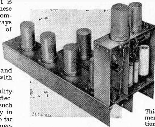
This photograph shows a development model of the receiver portion of the equipment. It comprises vision and sound R.F. channels and detectors together with the V.F. stage.
