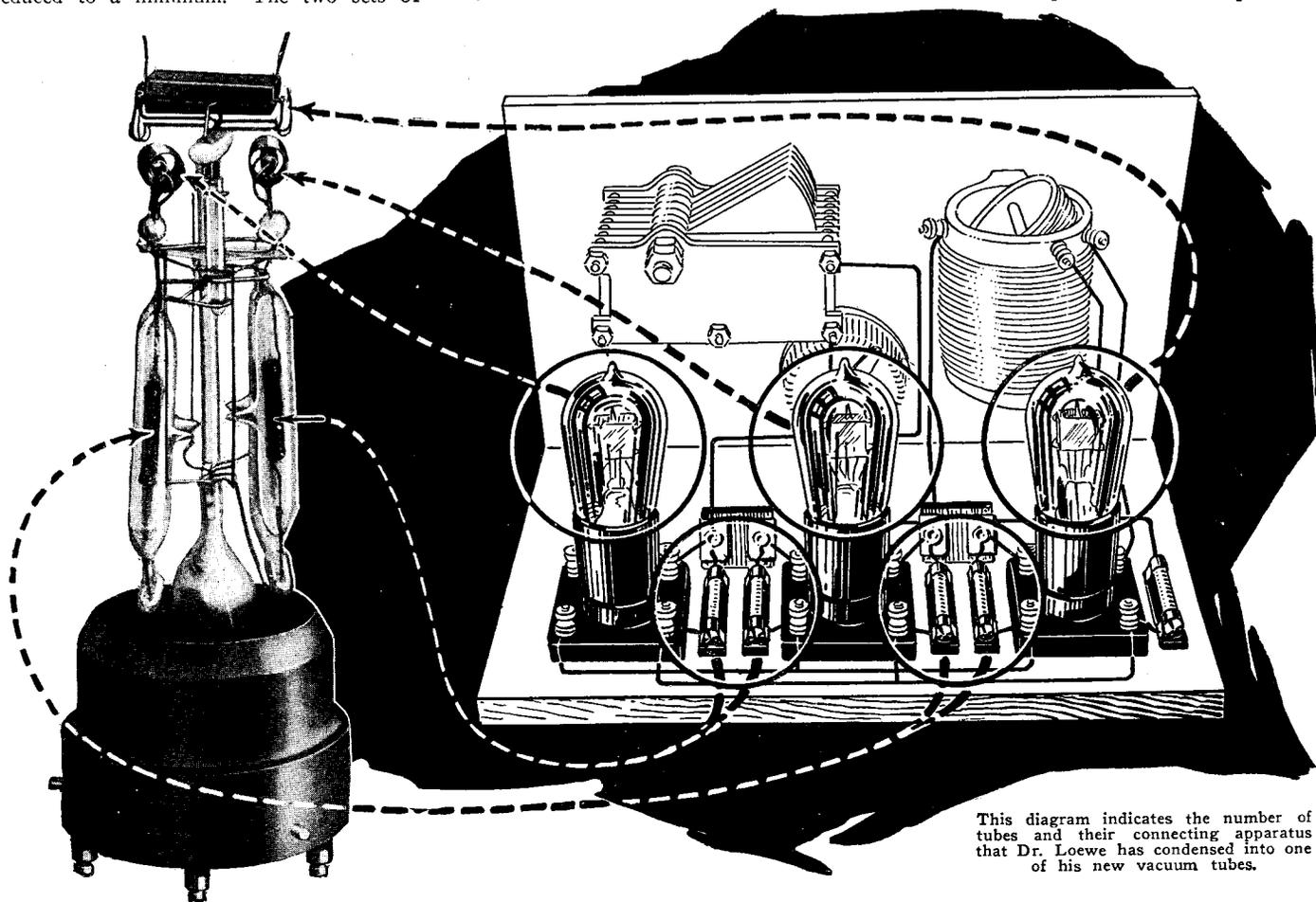
This diagram indicates the number of tubes and their connecting apparatus that Dr. Loewe has condensed into one of his new vacuum tubes.
