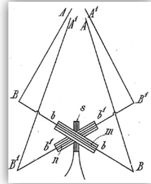
**Figure 5b (right):** Bellini's and Tosi's US 943,960 (1909) direction finding system used a fixed orthogonal DF array and a rotatable transformer for steering.
