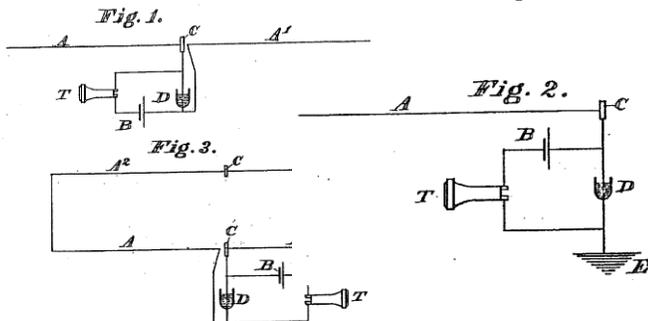
**Figure 4:** De Forest's US 771,819 (1904) rotatable direction finding antennas: a horizontal dipole (top-left), an "L" monopole (right), and a loop antenna (bottom-left).
