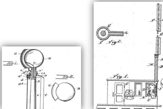
**Figure 1a (left):** Kitsee and Wilson's US 651,014 (1900) direction finding antenna relied on shielding of a spherical capacitive end load to "shadow" signals.
