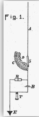
**Figure 5a (left):** De Forest's US 771,819 (1904) signal ranging apparatus employing a variable resistor to evaluate signal strength and correlate it to range.
