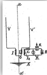
**Figure 3:** Stone's US 716,134 and US 716,135 (1902) direction finding antenna system.
