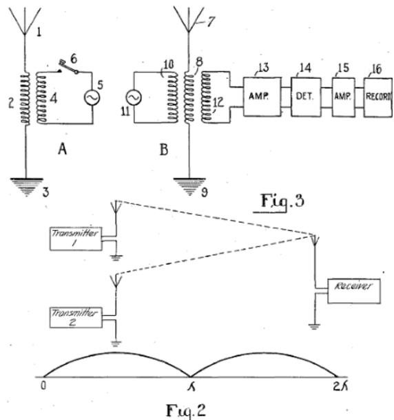
**Figure 7:** Ranger’s US 1,639,667 (1927) direction finding antenna system requires precisely synchronized oscillators at transmitter and receiver and determines distance from a starting point by counting the number of half wavelength beats in the rectified signal.
