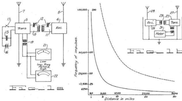
Figure 9 Nicolson's US 1,945,952 (1931) radio range finder employed standing waves, exploiting time-of-flight of a signal to a transponder and back to determine range.
