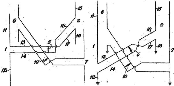
**Figure 6:** Two embodiments of Adcock’s GB 130,490 (1919) direction finding antenna system, a dipole version (left) and a monopole version (right). Adcock’s configuration minimized horizontal coupling to ensure accurate readings even in the presence of skywave signals at night.
