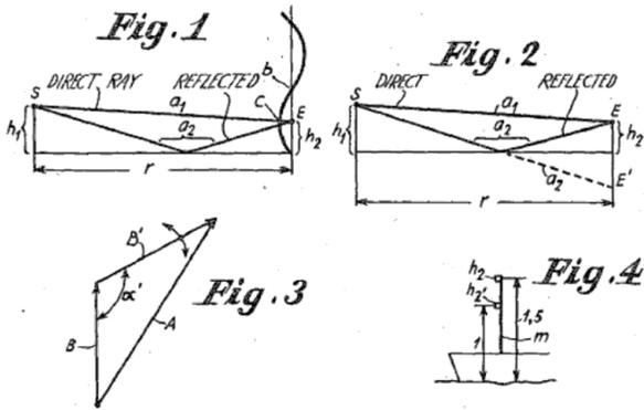
Figure 8: Runge's US 2,134,535 (1938) distance determining system employed the interference between direct and reflected signals as a navigational aid.
