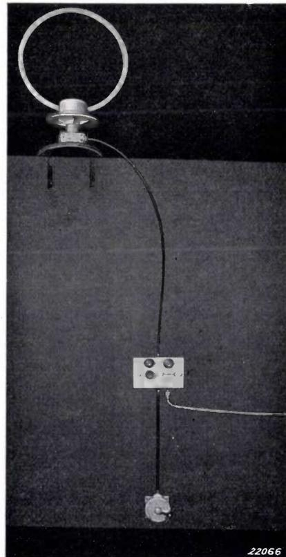
Fig. 4. Rotating loop aerial, angle indicator and arrangement for rotating the loop, for apparatus type V.P.K. 35.
