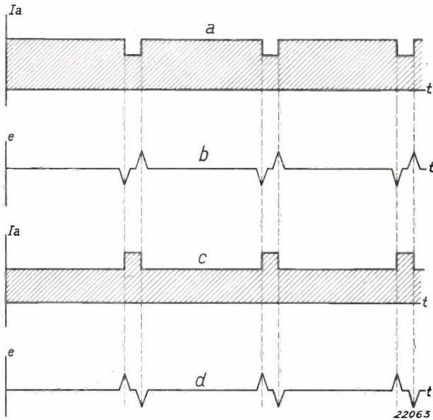
Fig. 6. Diagrammatic representation of the action of the visual indicator of the direction-finder homing-device, type V.P.K. 35.
