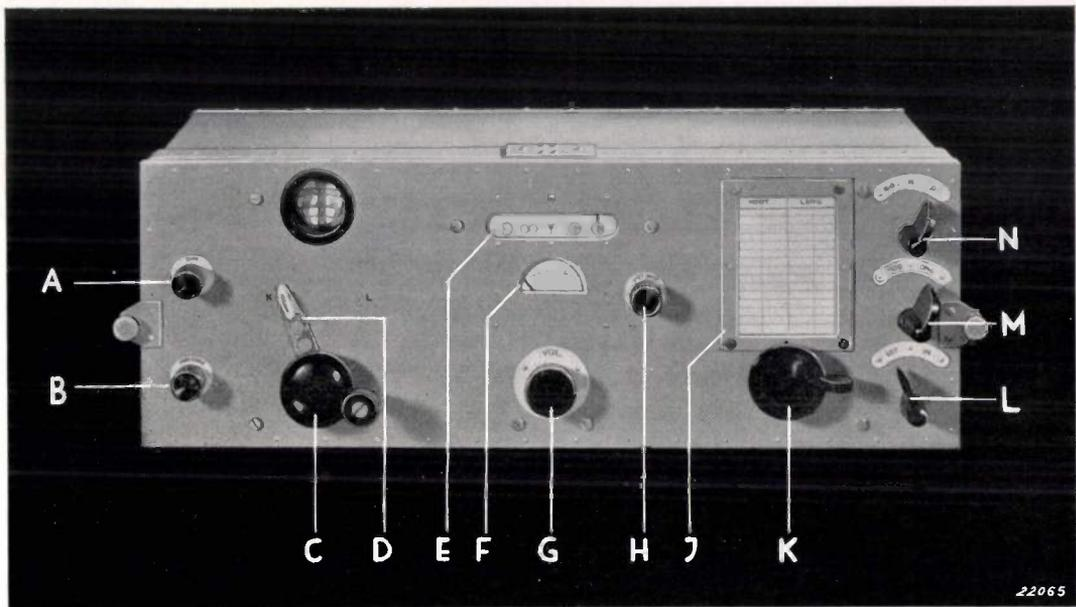
Fig. 3. Direction finder-homing device (Type V.P.K.P.. 35).
