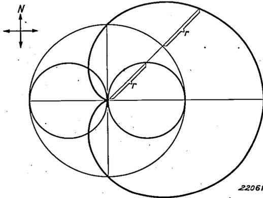
Fig. 2. Diagram of the receiving strength of a loop aerial (figure-eight shape) and non-directional aerial (circle). The heart-shaped diagram is obtained by combining these two in an appropriate way.
