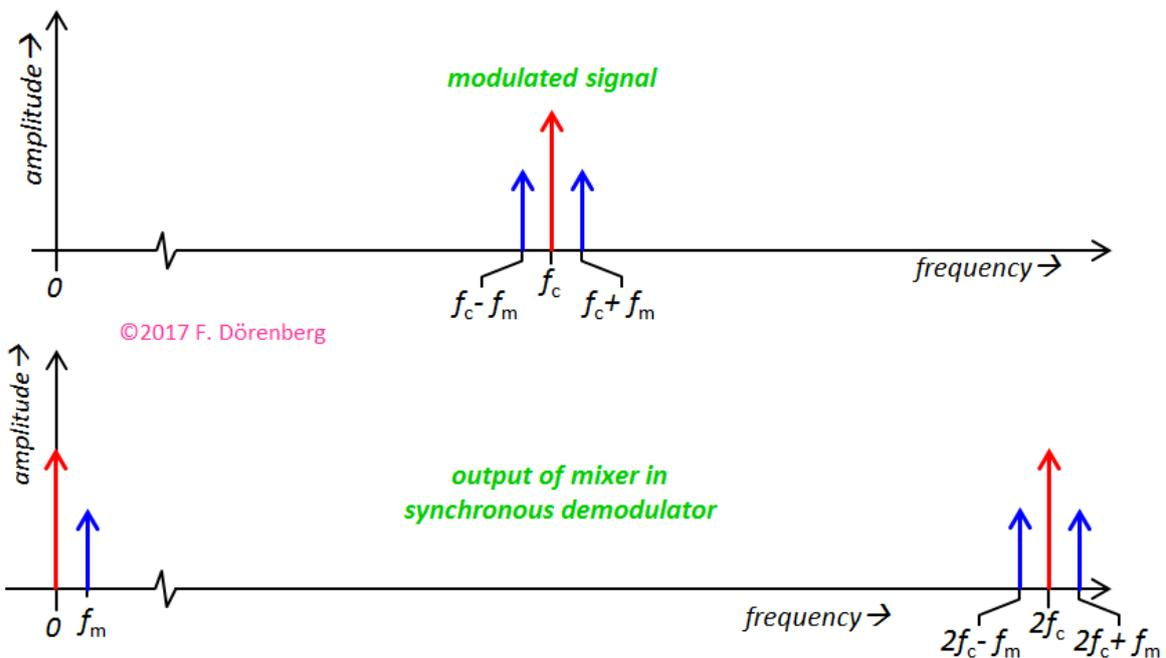
**Figure 4: AM modulation and synchronous de-modulation**
