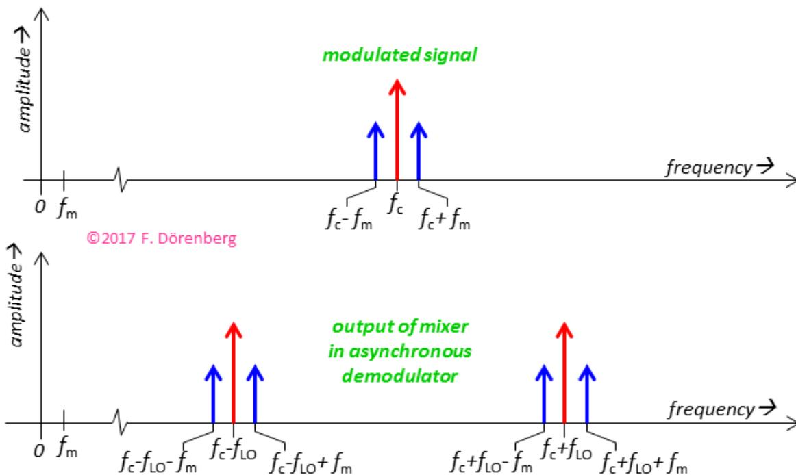
**Figure 5: AM modulation and asynchronous de-modulation**
