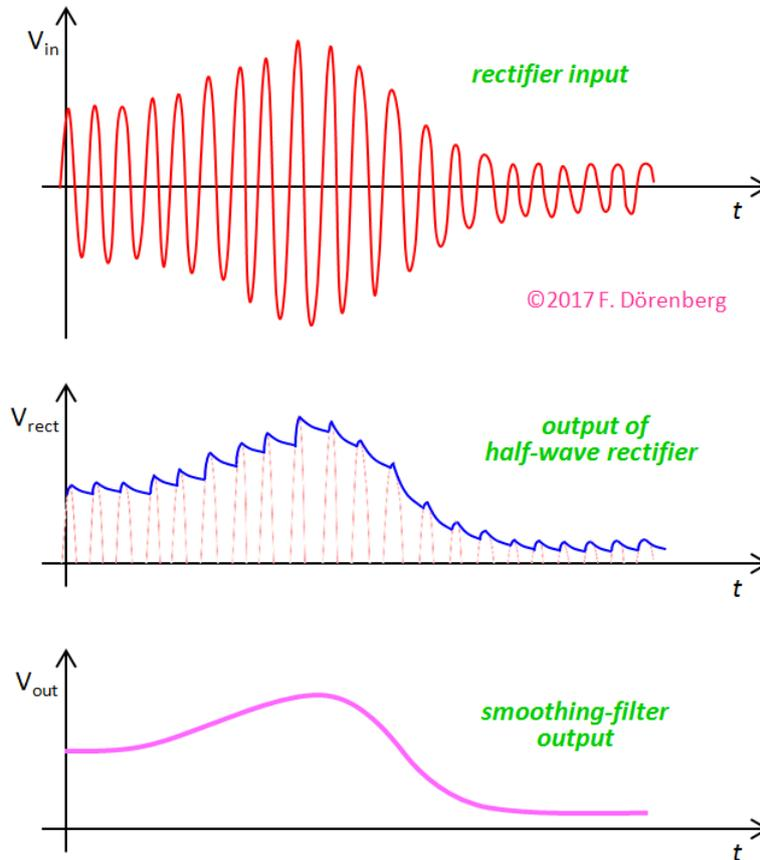
**Figure 3: input & output of a diode-rectifier envelope detector**
