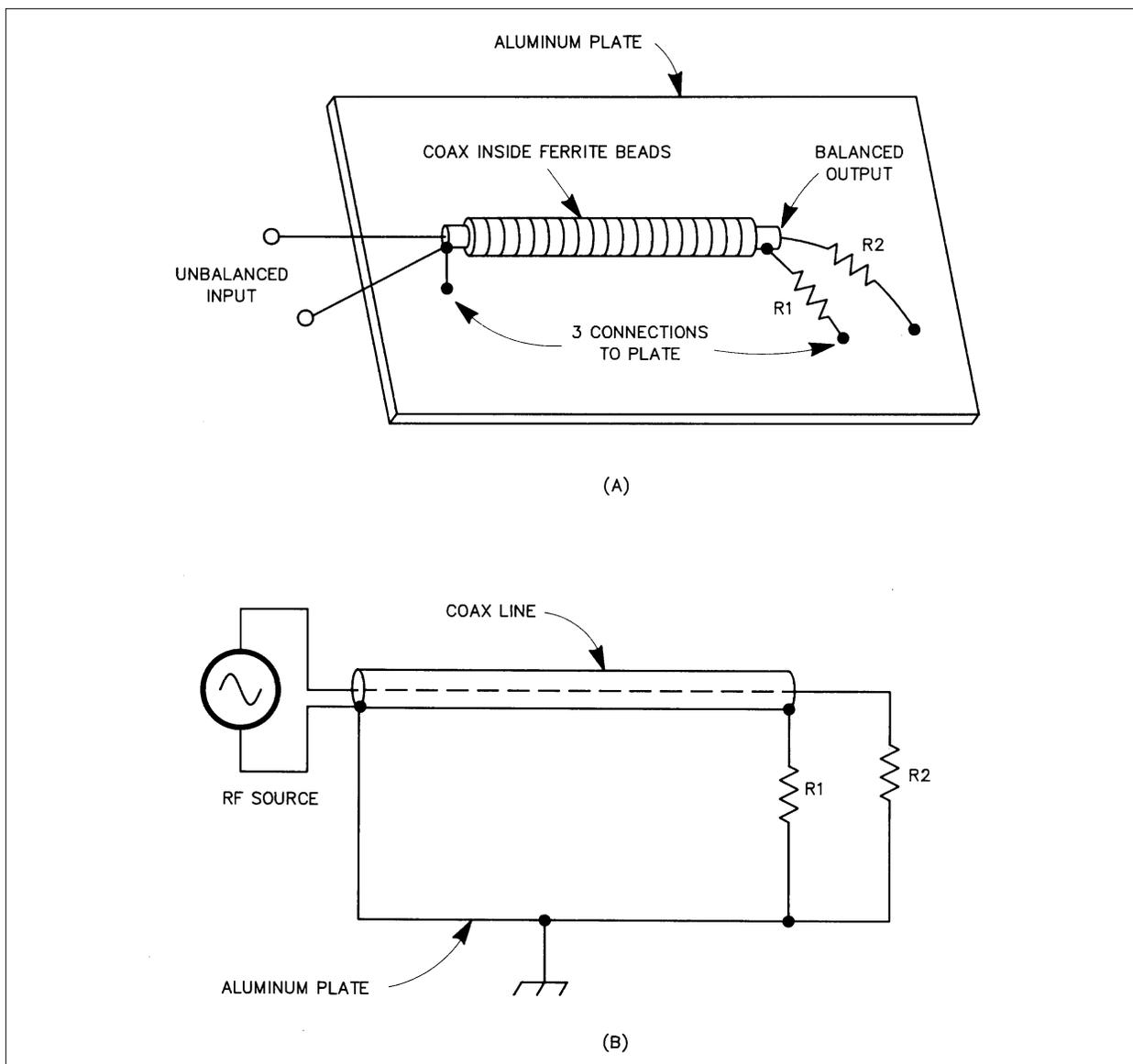
**Fig 21-4—The drawing at A shows a test setup for measuring the degree of balance in a current balun, and B shows its electrical equivalent, with an RF source. With a perfect balun and an RF voltage applied at the unbalanced input, the voltage drops across R1 and R2 will be directly proportional to their resistances. This proves that equal current flows in the two resistors, and no current flows on the outside of the coax shield to short out R1, contrary to the way it appears in B.**
