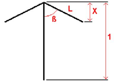
The influence of both effects depends of the number of topload wires, their length and their sloping angle. John Sexton (G4CNN) did develop a mathematical model for umbrella antennas with the goal to optimize the parameters (number of wires, length and sloping angle) for a maximum radiation resistance.
