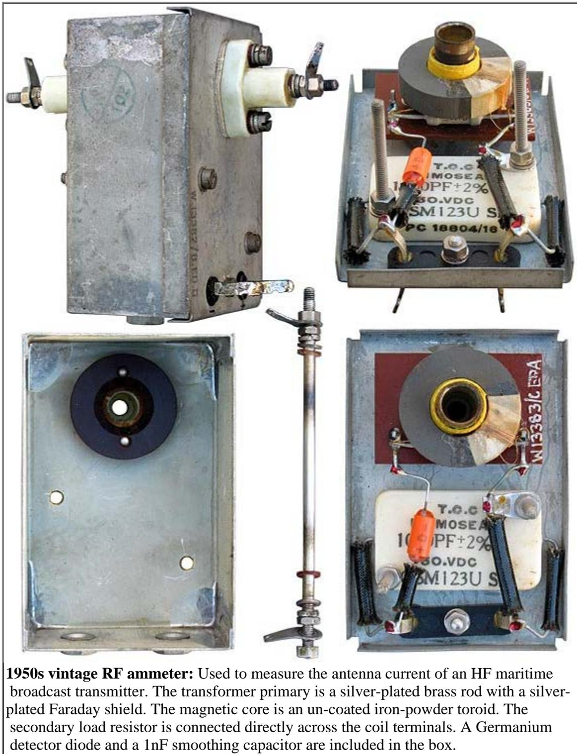
**1950s vintage RF ammeter:** Used to measure the antenna current of an HF maritime broadcast transmitter. The transformer primary is a silver-plated brass rod with a silver-plated Faraday shield. The magnetic core is an un-coated iron-powder toroid. The secondary load resistor is connected directly across the coil terminals. A Germanium detector diode and a 1nF smoothing capacitor are included in the box.
