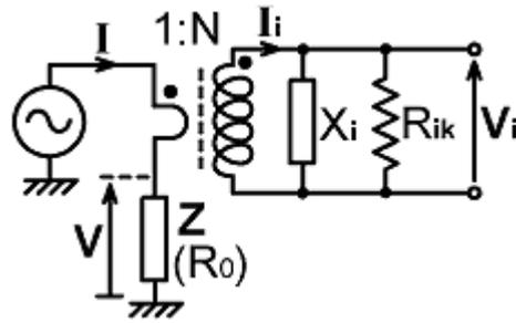
The balance point for a bridge is independent of the voltage or current associated with the primary load. Hence, when designing bridges, the use of dimensionless transfer functions preserves this independence. The design process then reduces to the matter of defining transfer functions for the current and voltage sampling networks and setting them to be equal when  $\mathbf{Z} = R_0$ . In that case, the transfer function for the current sampling network becomes:
