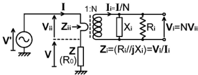
Using the definitions in the diagram, the input impedance or 'insertion impedance' of the primary is  $Z_{ii} = V_{ii}/I$ . Now note that  $V_{ii} = V_i/N$  and  $I = NI_i$ . Hence:
