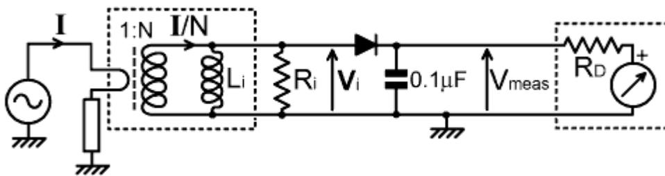
Here the detector is sensitive only to the magnitude of the output voltage, and the reading on the meter (assuming a scale calibrated to allow for diode forward voltage drop) is given by:
