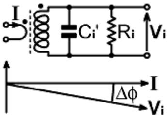
The phase shift depends on the load resistance and is given by:
