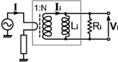
Here the capacitance has been ignored, and the inductance  $L_i$  should be taken to be about 1 or 2% less than the measured inductance of the secondary coil. The relationship between primary current and secondary voltage (neglecting losses) given earlier as equation (4.1) is now reduced to:
