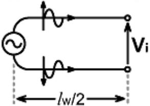
The two waves combine at the terminals to produce a finite output voltage because they cause opposing displacements of the potentials at the terminals.
