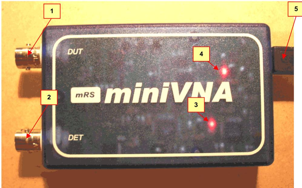
1. BNC DUT: rf out / antenna. **WARNING! Do not connect to RF transmitter**
