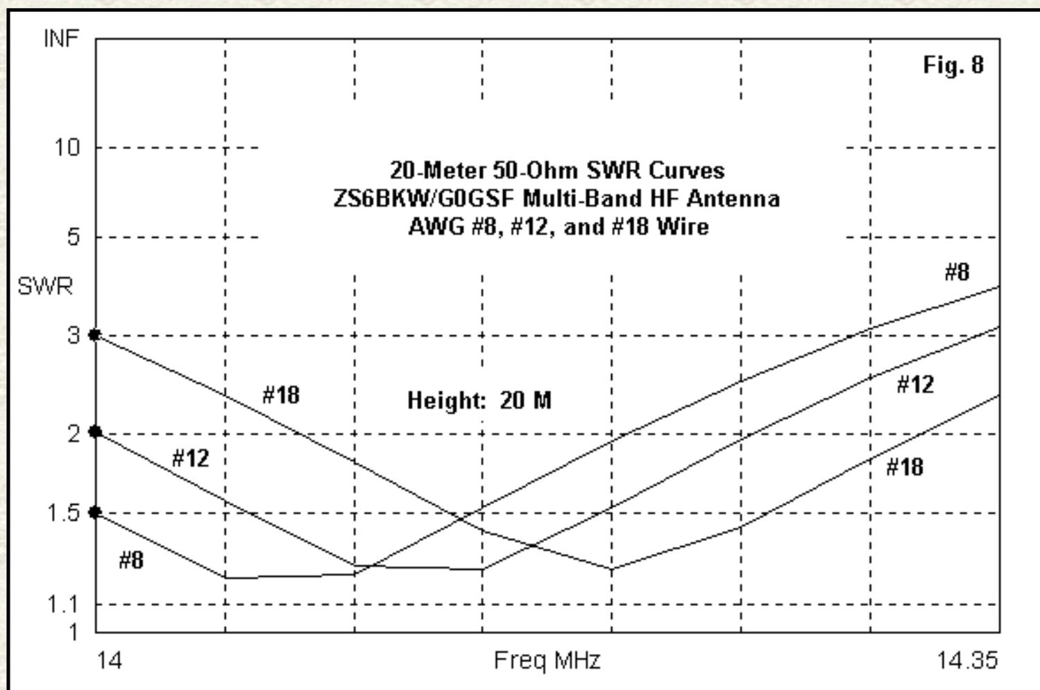
See **Fig. 8**: on 20 meters, as the operating bandwidth narrows, the thinner end of the wire scale offer fuller band coverage, with the #18 wire favoring the upper end of the band. Those who use only the low end of the band for CW or digital work might prefer a larger diameter wire for the antenna.
