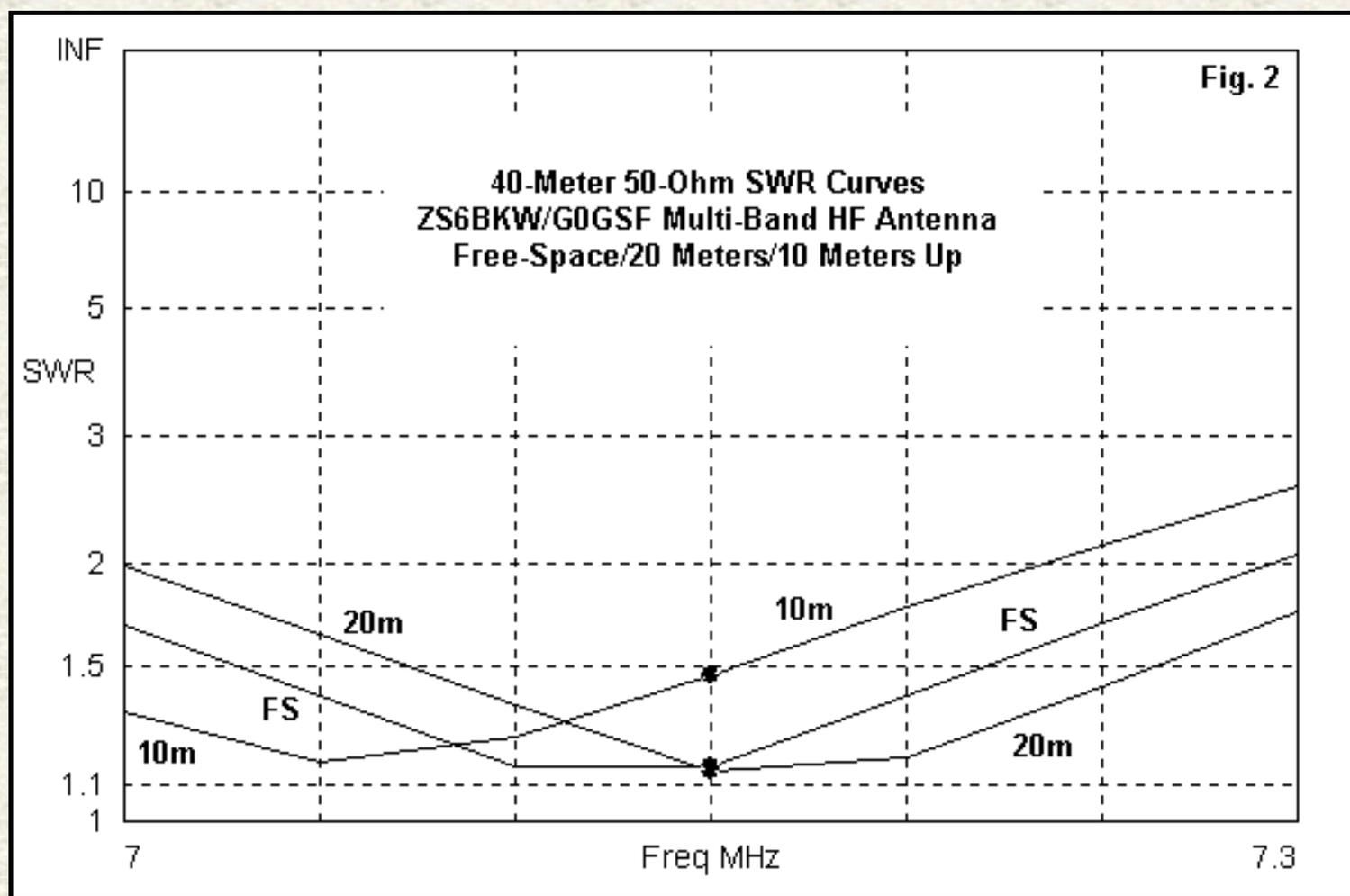
**Fig. 2** provides us with a triple sweep of 40 meters. Only the curve for the 20-m height covers the entire band with an acceptable (less than 2:1) 50-Ohm SWR. On 40 meters, that height is about 1/2 wavelength up, while the lower 10-m height is only a quarter wavelength.
