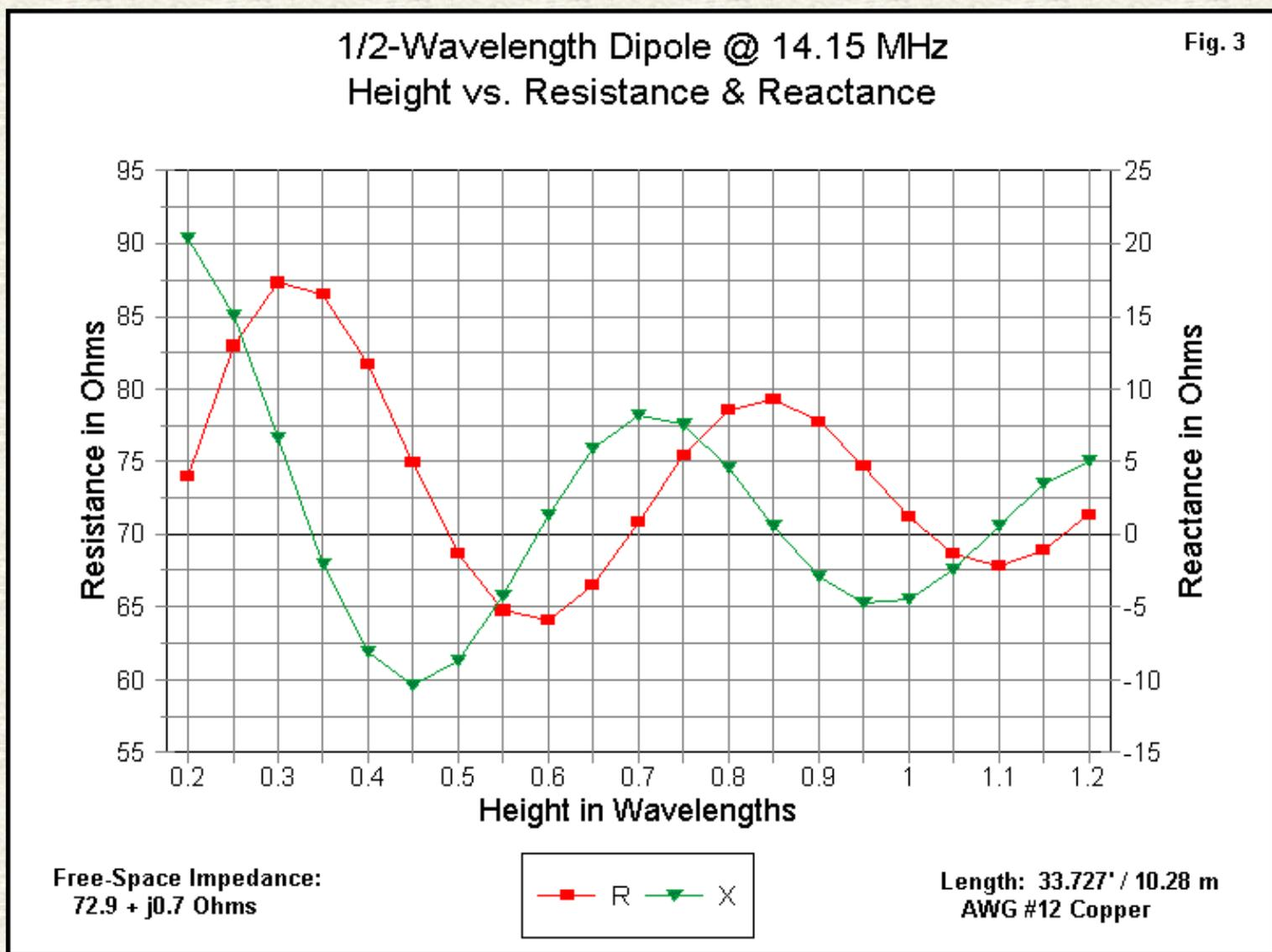
As noted earlier, the resistance and reactance cycles peak at 0.5-wavelength intervals of height. However, the resistance and reactance curves are not synchronized. The reactance peaks occur about 0.15-wavelength higher than their closest resistance peaks.
