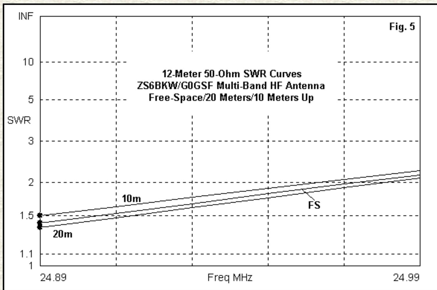
12 meters (**Fig. 5**) shows a similar phenomenon where the 50-Ohm SWR passes the 2:1 mark within the band. However, for most heights, the SWR is a bit lower than on 17, and the same length of coax would show a bit more loss and hence a bit lower SWR at the transmitter end of the line. Hence, the 12-meter band might prove a bit less problematical relative to triggering power reduction circuitry.
