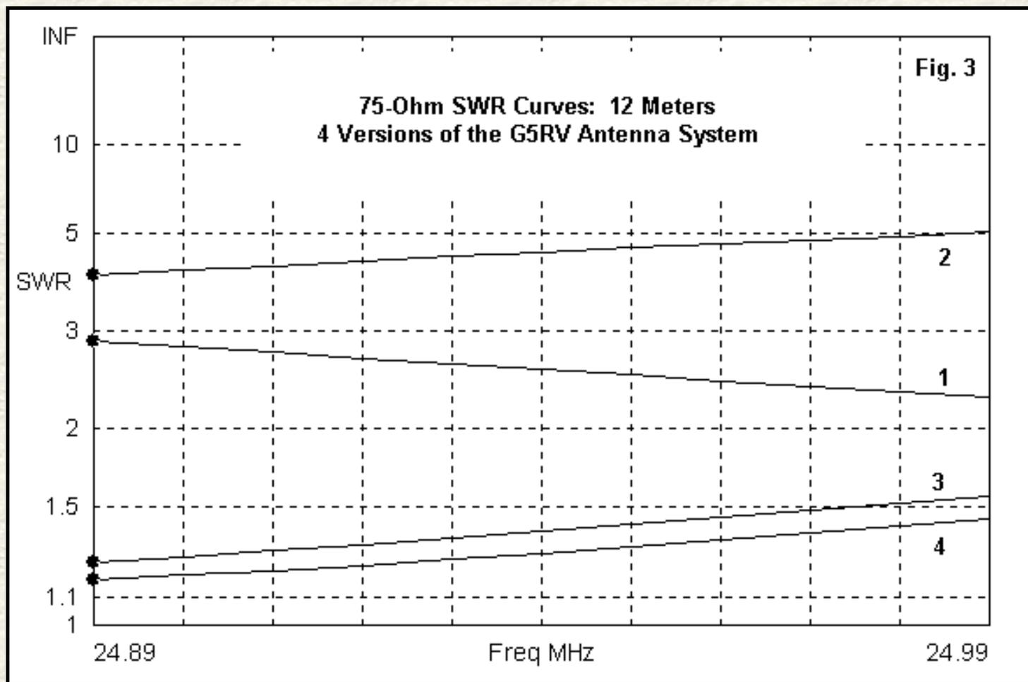
As may be evident, the two 300-Ohm systems provide a good 75-Ohm SWR, while the two higher-impedance matching sections do not. The unsuspecting novice builder of a G5RV may wonder why.
