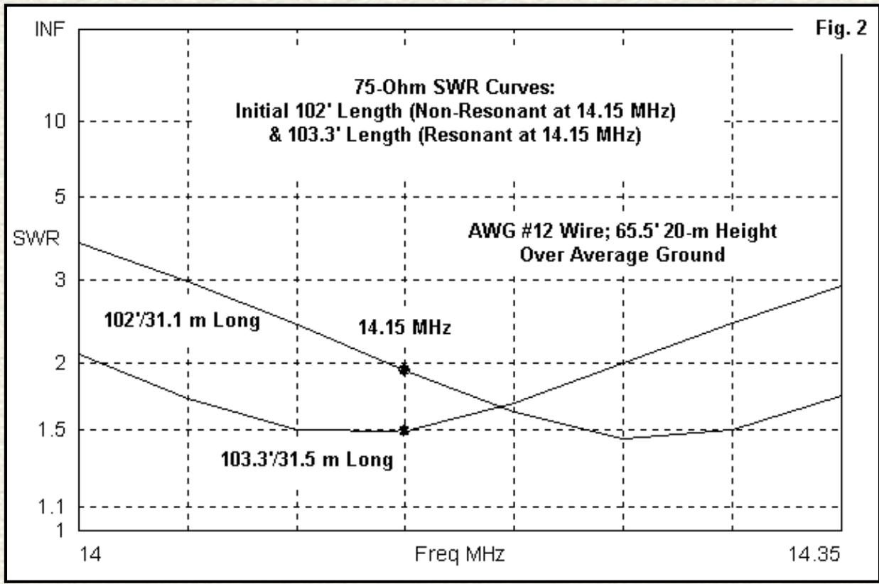
**Fig. 2** shows the curves for the short and the long antennas. Clearly, the longer length favors the lower end of 20 meters, while the 102' length favors the upper end of the band. The impedance level of a G5RV is high enough that we cannot obtain full band coverage from the wire and line combinations. In addition, the 1/2-wavelength line section is 1/2 wavelength only at the design frequency. Hence, it contributes to a narrowing of the SWR bandwidth.
