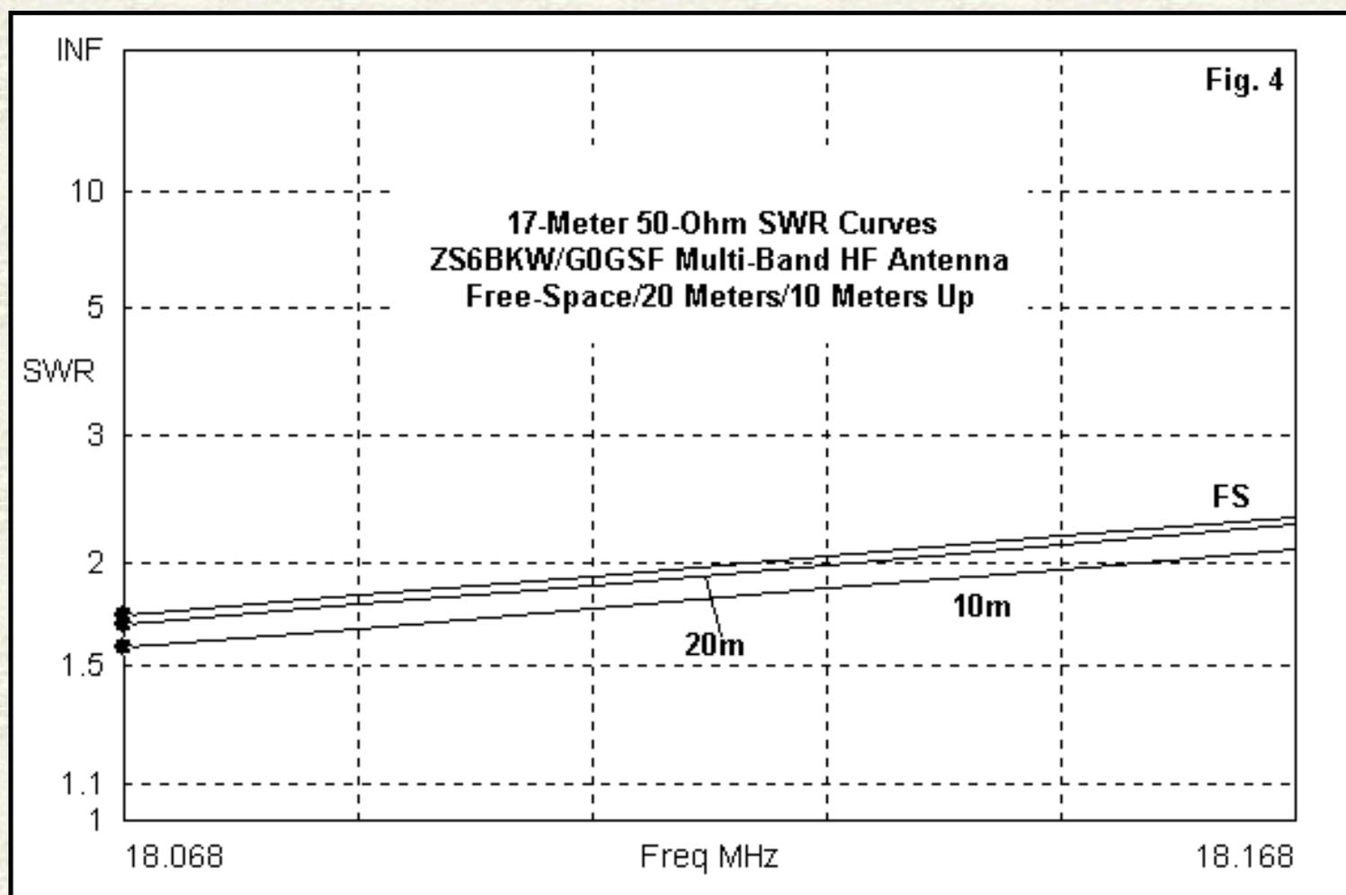
The 17-meter band is marginal with respect to a 2:1 SWR bandwidth, as shown in **Fig. 4**. With a length of 50-Ohm coax between the matching section and the rig, the measured SWR near the transmitter would be a bit less, allowing the use of this band without triggering most power-reduction features associated with solid-state final amplifiers.
