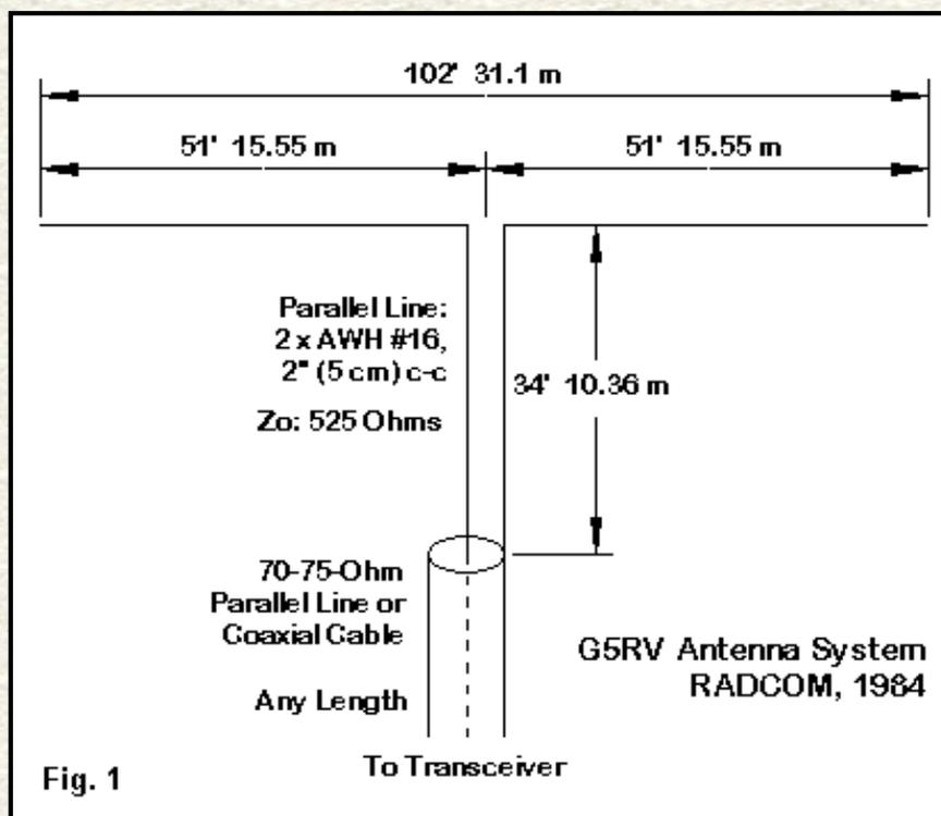
However, we conventionally sketch the G5RV antenna system as in Fig. 1. The center-fed doublet has a section of parallel transmission line extending from the radiating wire feedpoint to a junction with the "main" feedline.
