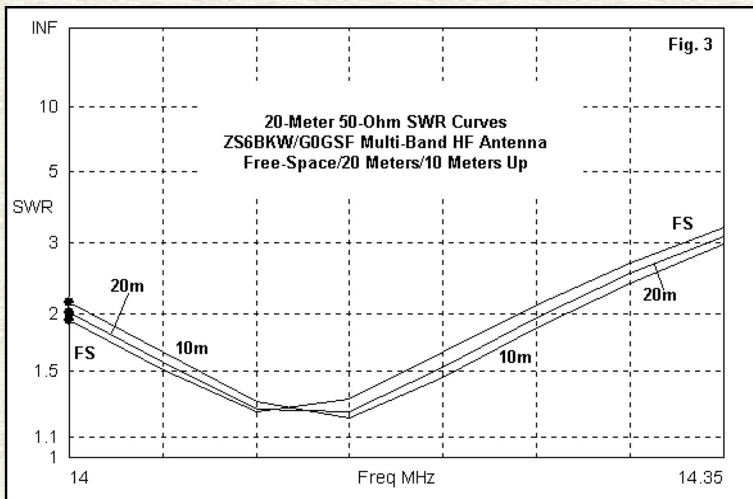
The 20-meter curves, shown in **Fig. 3**, coincide more closely, since the heights are 1/2 and 1 wavelength. The SWR bandwidth favors the low end of the band and is narrower than would be the SWR curve for an AWG #12 copper dipole resonated somewhere in the middle of the band.
