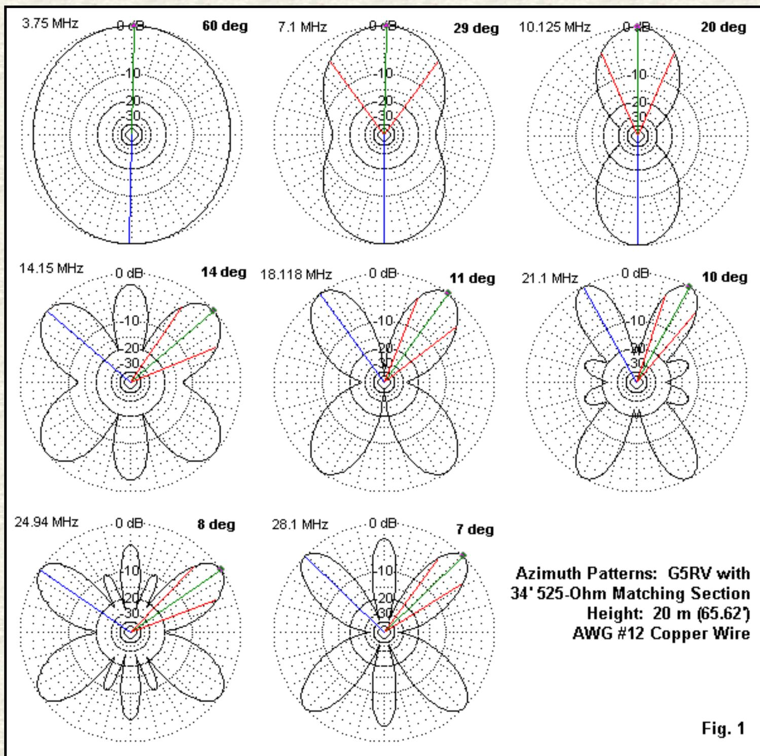
Each pattern in **Fig. 1** shows the frequency at which it was taken, along with the TO angle. 102' represent a little over 1 wavelength at 10.125 MHz, and so we see two broadside lobes. The antenna is about 2 wavelengths long at 17 meters, revealing a 4-lobe pattern. At 10 meters, the antenna is close to 3-wavelengths long and shows 6 distinct lobes.
