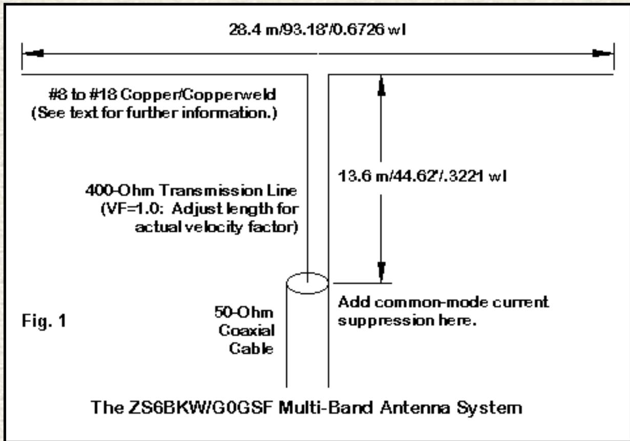
**Fig. 1** shows the outline for a ZS6BKW/G0GSF antenna system for 40 through 10 meters. The wire length is 28.4 m or 93.18'. The matching section uses 400-Ohm parallel line and a length of 13.6 m or 44.62'. We shall examine various wire sizes for L1 later, but for the moment we may note the following small table of values for constructing 400-Ohm open wire transmission line using common copper wire sizes.
