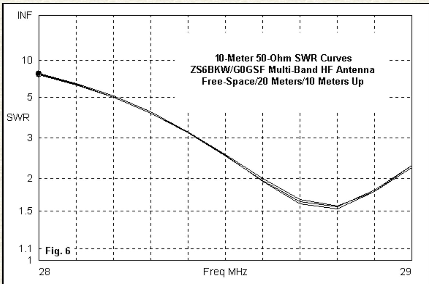
Because the "good-match" frequency ratios are not harmonically related, the ZS6BKW/G0GSF antenna system favors the upper end of the first MHz of 10 meters, as shown in **Fig. 6**. The window is small, but quite usable. If the transceiver has a built-in narrow range tuner, of course, the entire band would be usable, and the marginal and narrow band conditions on other bands would no longer be a problem.
